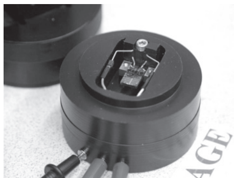
Figure 4.5: The new sample holder for HECL measurements. A silicon HECL chip with a PDMS lid is shown inserted into the holder. The two front side contacts and the substrate contact are wired to the three terminals in the holder base. A separate photomultiplier tube assembly fits over the sample holder.
